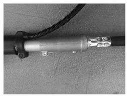
CAUTION: If the flexible tube is not inserted properly, the square end of the hose may not fit snugly in the drive shaft seal. Do not use force to avoid damage to the flexible shaft. Repeat the same procedure until the flexible shaft and hose are adjusted.
